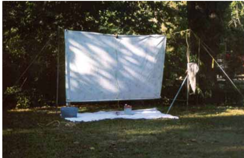
Figure 11: Lite trap set up for demonstration. A small battery powered light is placed atop a vertically strung sheet that lies perpendicular to a ground sheet.
